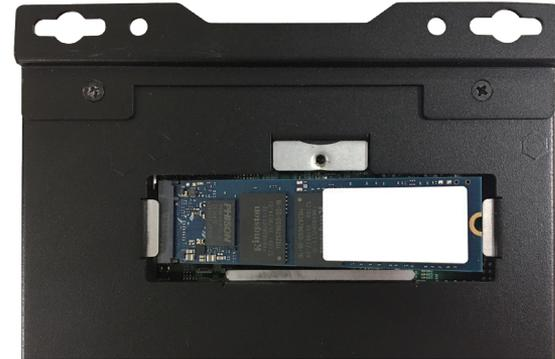
3. Once the module has been fully inserted, tighten the screw into the mounting hole to secure it in place.
