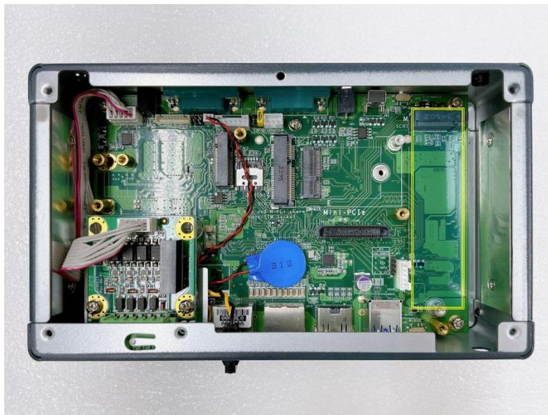
**Step 4** Take the SSD thermal bracket, four thermal pads, and two M3 screws out of the package box.
