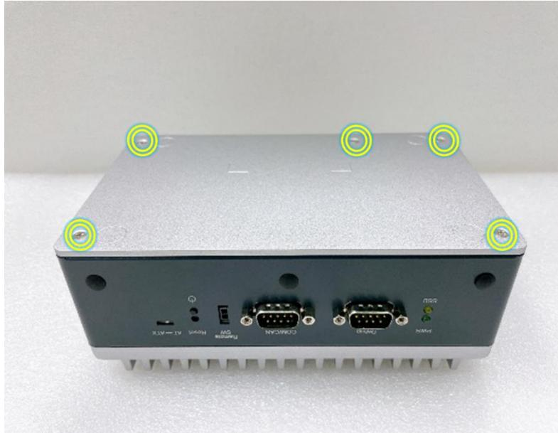
**Step 3** Remove the bottom cover, and locate PCI Express mini card slot on the board.
