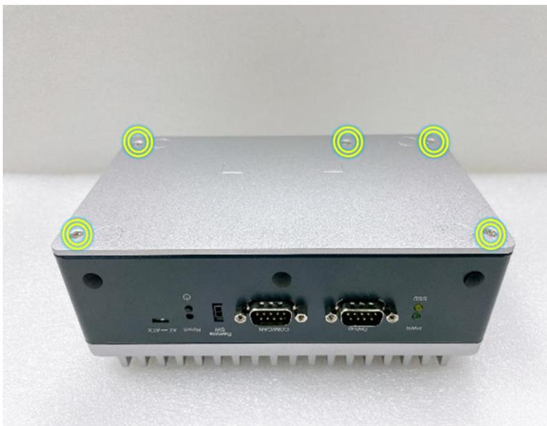
**Step 4** Take off the bottom cover, and locate the M.2 2230 Key E slot on the carrier board.
