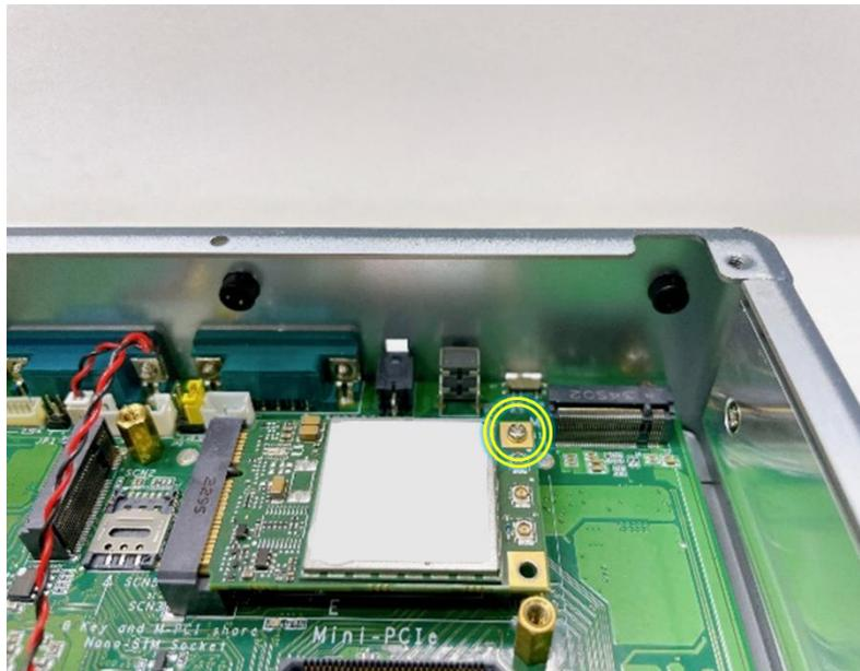
**Step 6 Connect the SMA cables to the PCI Express mini card.**
