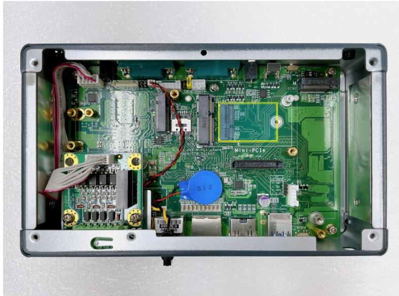
**Step 5** While holding the M.2 Key E 2230 module at a 30 degree angle up from the horizontal, slowly insert the golden fingers into the M.2 Key E 2230 slot, until it is fully inserted in place.
