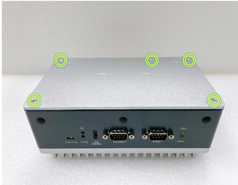
**Step 3** Take off the bottom cover, and locate the M.2 2280 Key M slot on the board.
