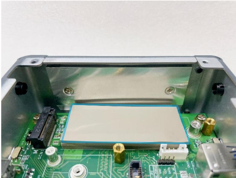
**Step 7** While holding the M.2 2280 Key M SSD drive at a 30-degree angle up from the horizontal, slowly insert the golden fingers into the M.2 2280 Key M slot, until it is fully inserted in place.
