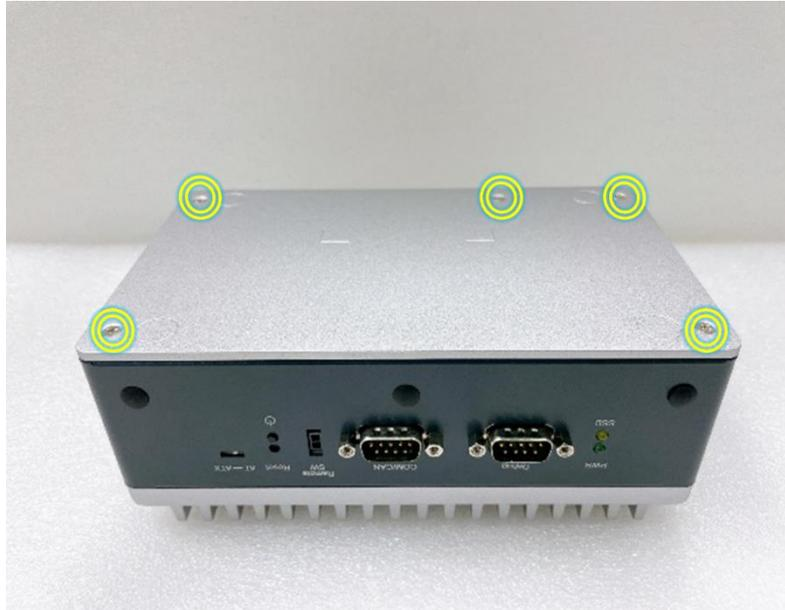
Step 3 Take off the bottom cover, and locate the M.2 3042/3052 Key B slot on the carrier board.
