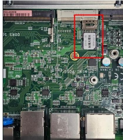
**Secure the SIM card by sliding the holder**
