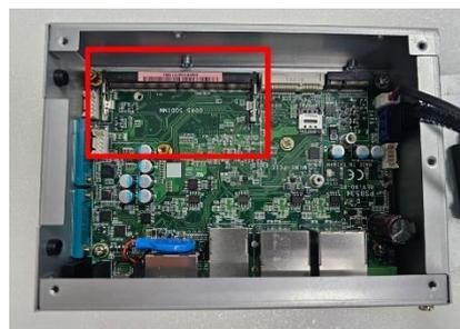
**Step 4** Insert the SO-DIMM into the socket and push the module down until it is locked in place by the two end latches.
