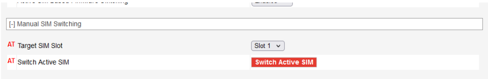
Figure 4-7: ACEmanager: WAN/Cellular > Cellular > General (Dual SIM settings)
