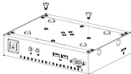
**Step1.** Insert and fasten two M3\*L11.1 screw on the bottom.
