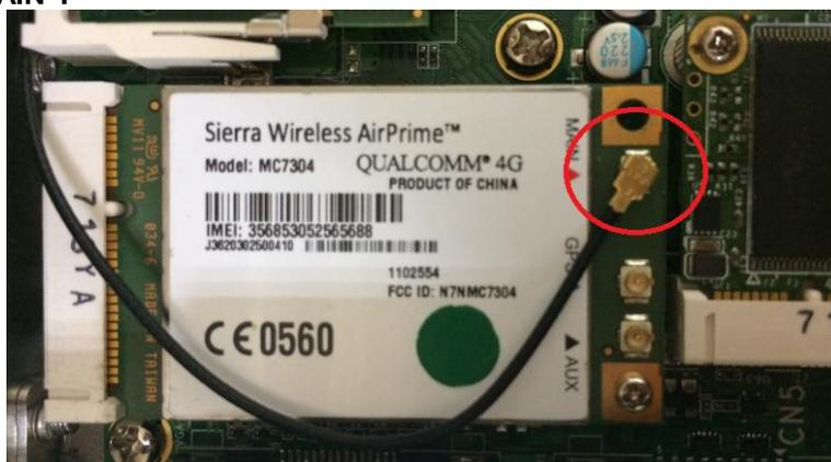
**Step 8** Taking out the parts from the 3G kit package (Figure 8-1) and make the RF cable through the antenna hole (Figure 8-2). Finally, screw it tight(Figure8-3).
