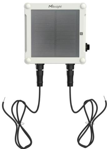
UC51x series LoRaWAN® wireless solenoid valve controller is a device used to remotely control DC latching solenoids of the valve. It contains 2 solenoid interfaces and 1 pulse interface, which can be easily controlled locally or remotely.
