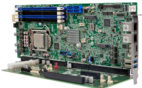
Standard PICMG 1.3 SBCs have several advantages over non-standard SBCs. Firstly, they are more maintainable than a motherboard system and have a much lower mean time to repair (MTTR). Secondly, it is easy to upgrade to a newer or faster processor if desired.
