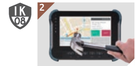
External damage protection
