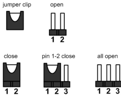
Properly configure jumper settings on the CAPA840/843 to meet your application purpose. Below you can find a summary table of all jumpers and onboard default settings.
