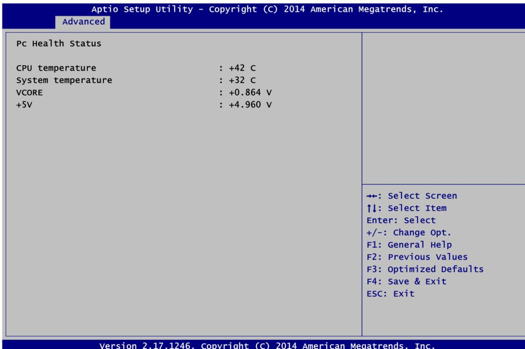
This screen displays the temperature of system and CPU, system voltages (VCORE and +5V).
