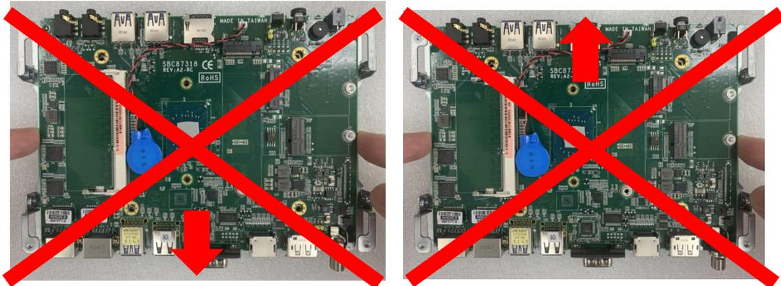
**Step 6** Flip the main board over and locate the DIMM socket on the back side of the board.
