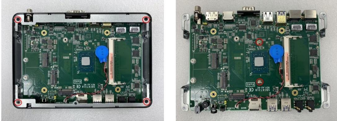
**Step 5 Carefully remove the main board away from the back cover underneath, as instructed below:**
