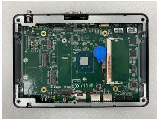
**Step 4** Locate the DIMM socket on the main board.
