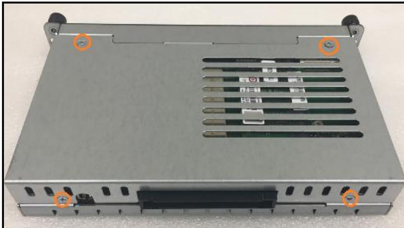
**Step 2** After losing the screws, extract the rear of chassis out of the module.
