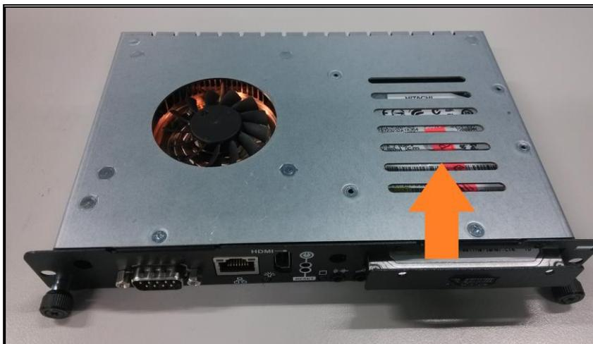
**Step 4** Finally, fasten two screws on HDD cover firmly to complete installation.
