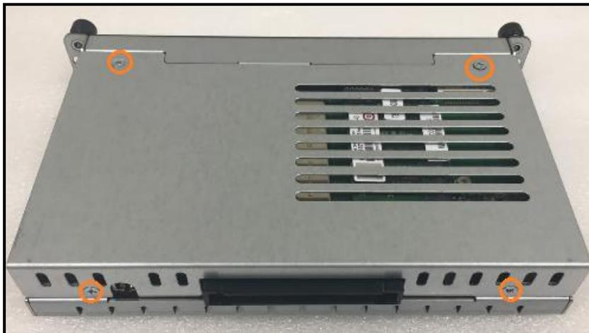
**Step 2** After losing the screws, extract the rear of chassis out of the module carefully.
