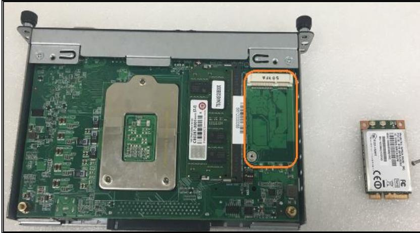
**Step 4 Please insert the module then fasten screw carefully.**
