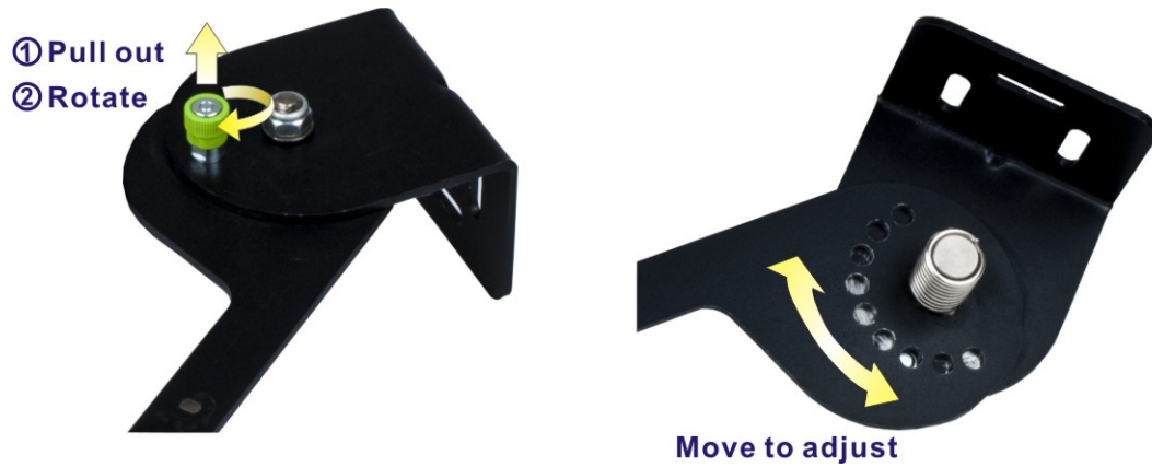
Figure 3-20: Ceiling Mounting Bracket Adjustment
