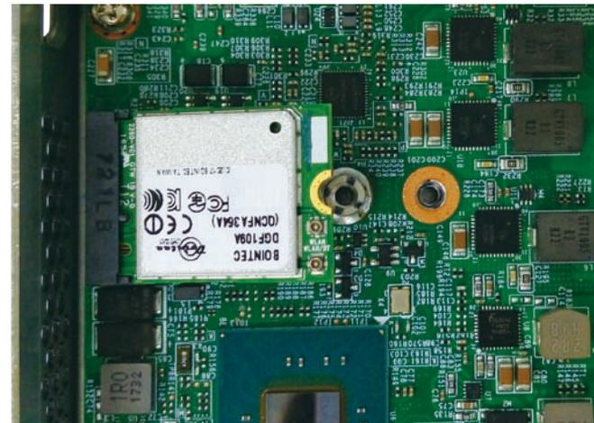
3. With the module fully inserted, tighten a screw into the mounting hole on the module to secure it.
