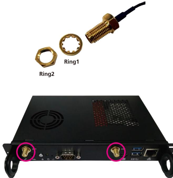
6. Connect the external antennas to the Wi-Fi antenna jacks.
