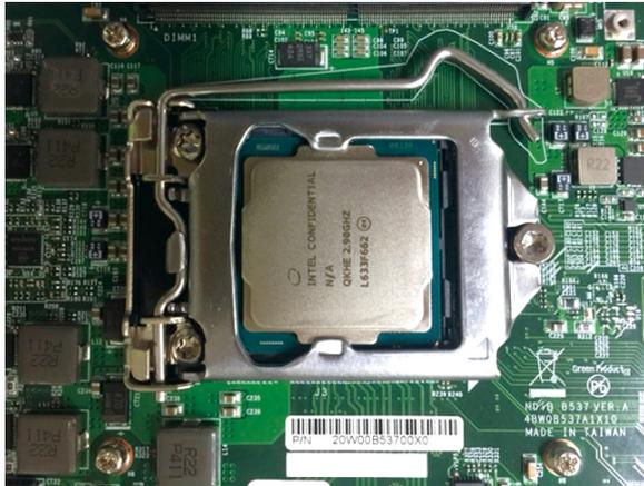
5. Remove the adhesive film on the thermal pad and place it onto the CPU.
