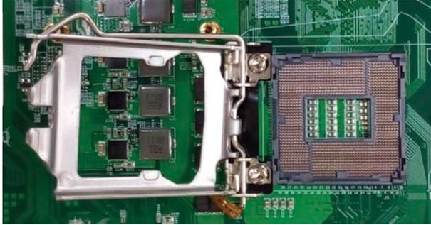
3. Insert the CPU into the socket. The triangular edge on the CPU must align with the corner of the CPU socket shown on the photo.
