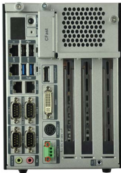
Figure 3-9: Pluggable DC-in Terminal Block Installation
