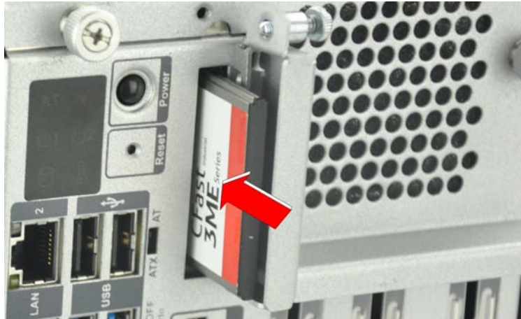
Figure 3-3: CF Card Installation
