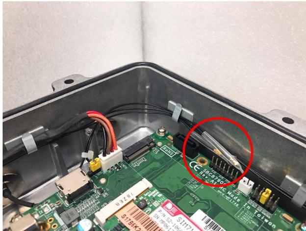
**Step 7** Connect the SMA cables to I-PEX connector of LTE Module and install LTE Antennas. And please do not place antenna cables on the top of PCI Express mini card, in case the SMA cables would loose.
