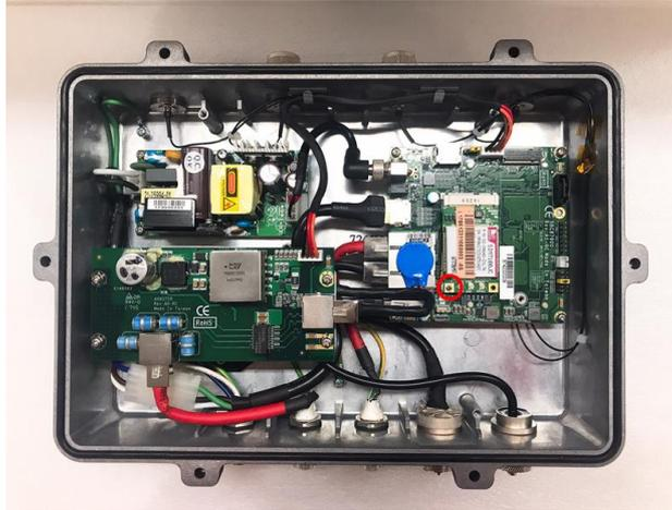
**Step 6** Find the SMA cables from the adhesive backed cord clip attached at the chassis as picture below.
