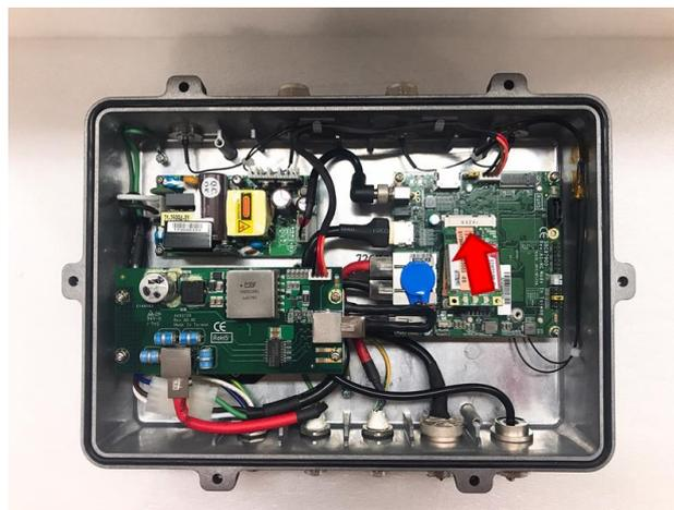
**Step 5** Press it down gently, but firmly, and then secure the PCI Express mini card to the carrier by tightening up the one M2\*5L screw to the marked position.
