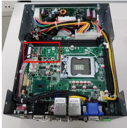
**Step 5** Slide Mini Card into Mini Card slot with caution, and fasten screw of Express Mini Card.
