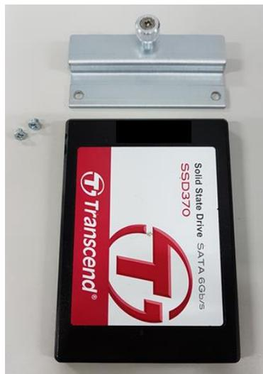
**Step 5 Fasten two screws to fix SSD/HDD.**
