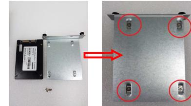
**Step 5** Connected the SSD directly and make sure the insertion is complete and fasten two screws.
