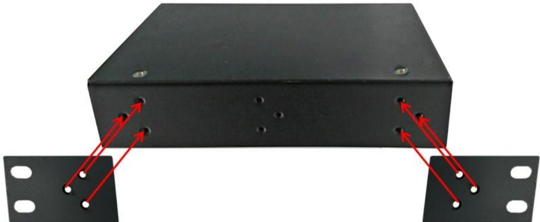
4. Use the hook holes at the corners of the wall-mount plates to hang the industrial switch on the wall.
