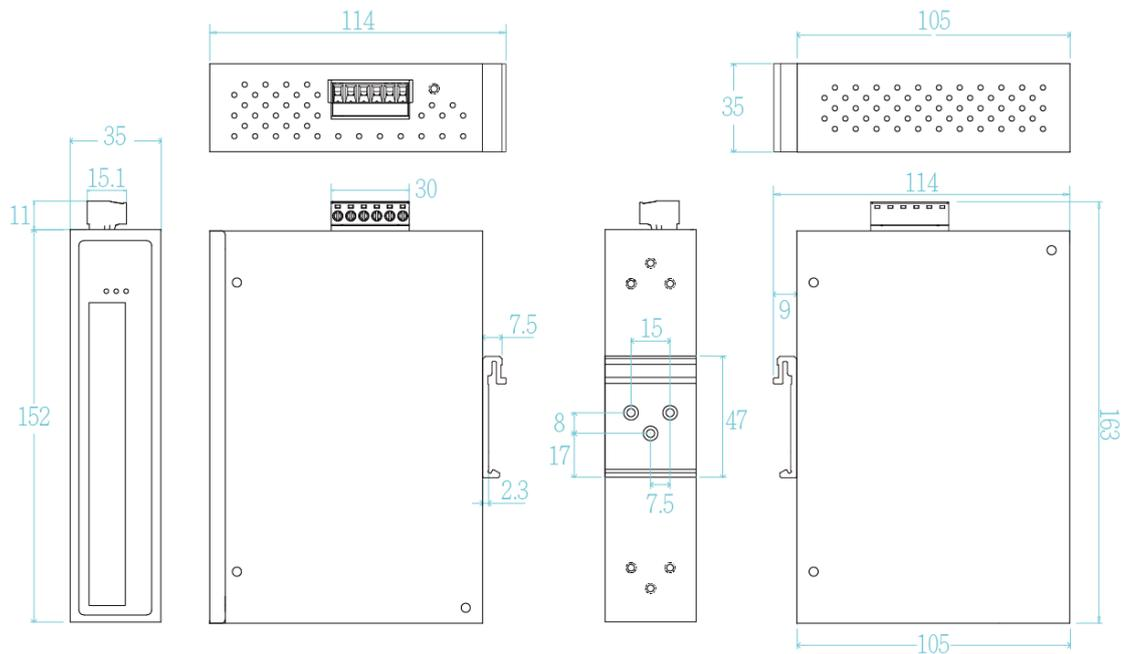
The dimensions of IPGS-0008B/IPES-0008B are 43 x 152 x 105 mm (W x H x D). The figure below gives the dimensions and views of each side of the 8-port 10/100/1000Base-T Industrial Switch.
