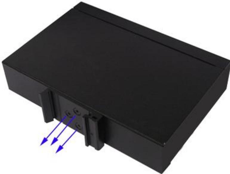
2. Place the wall-mount plates on the rear panel of the industrial switch.
