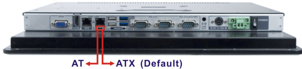
Figure 3-21: AT/ATX Mode Selection
