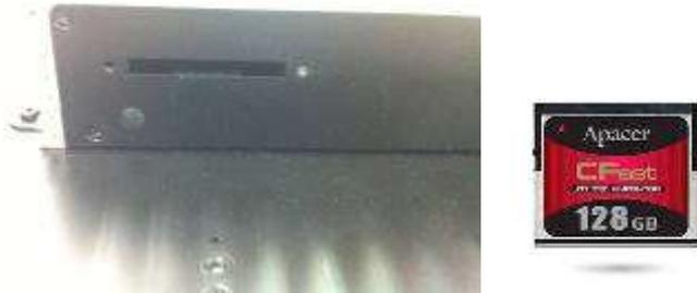
**Step 3** Insert the CFast card to the CFast card slot, then finding the CFast cover and screw it.
