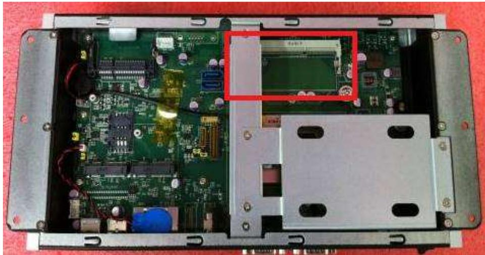
**Step 3** Insert the DRAM to the DIMM socket, and then push it down firmly until it is clipped by the socket. Installation completed
