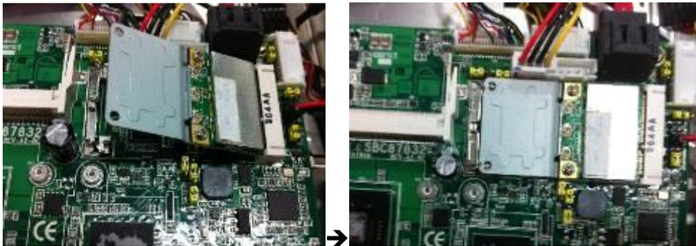
**Step 3** Find the Antenna cable and connect it on wireless LAN card.
