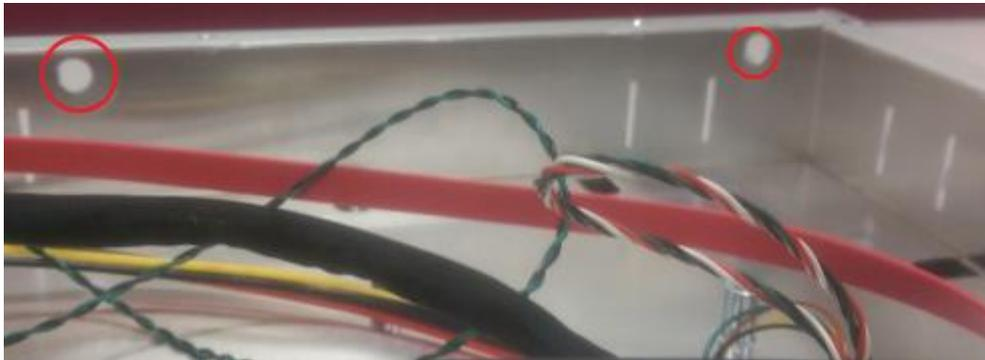
**Step 4** Remove the antenna plug from the top of back cover, then Install the antenna on the antenna connector.
