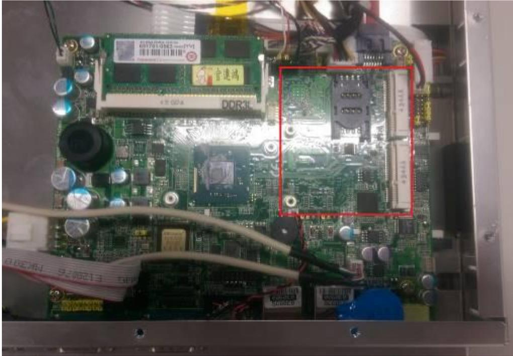
**Step 2** Insert the wireless LAN card to the slot. Push it down firmly until it is clipped by the slot.
