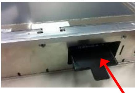
**Step 4** Close the cover of CFast™ card slot and fix it. Installation completes.
