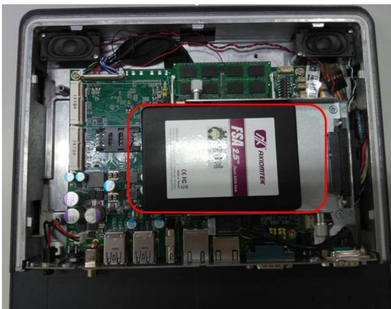
**Step 4 Screw the 2.5" SSD/HDD to fix SSD/HDD.**
