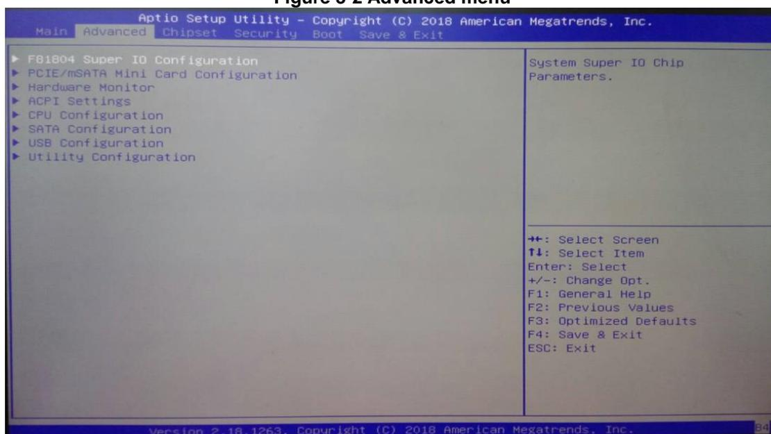
The Advanced menu allows users to set configurations of the CPU and other system devices. Select any item on the left to go to the sub-menus (as shown in Figure 3-2).
