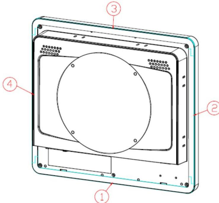
**Step2** Assemble the panel kit to the chassis and fix the six screws
