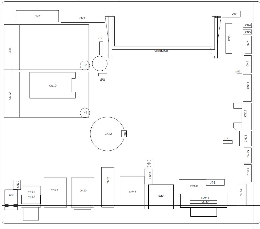
Diagram 2-2 Solder side of the board
