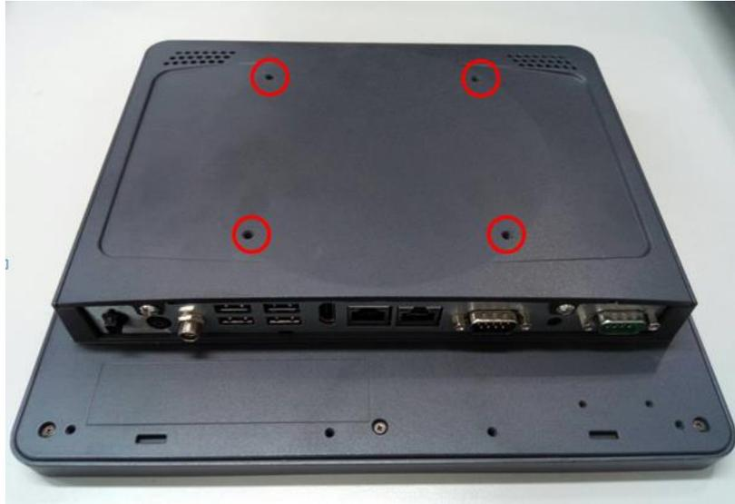
**Step 2** Assemble the wall mount bracket to the back side of the chassis, and fix the screws.
